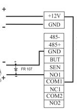
Device share power with the lock: ULOCK=12V, I-ILOCK>1A······ (1) And the lock is near to the device.
